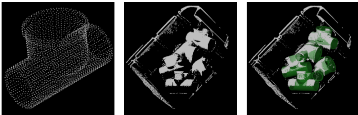
Figure 1.1: The surface model of an object (left), a 3D point cloud (center), where the surface model should be located in, and the final matching result (right), where the found instances of the model are marked green.
