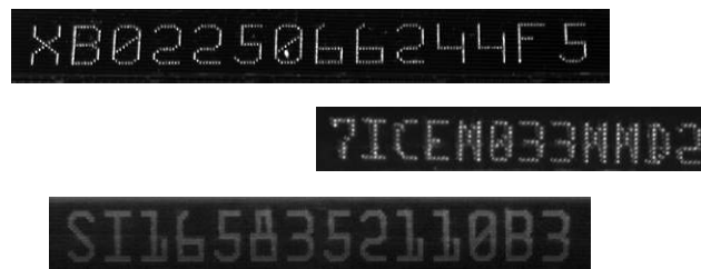
Figure 18.20: Examples for SEMI font. Note that these images were inverted before the training was applied! That is, this font is nevertheless pretrained only for dark on light symbols.
