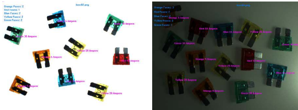
Figure 14.6: Simple classification of fuses by color with varying illumination.
