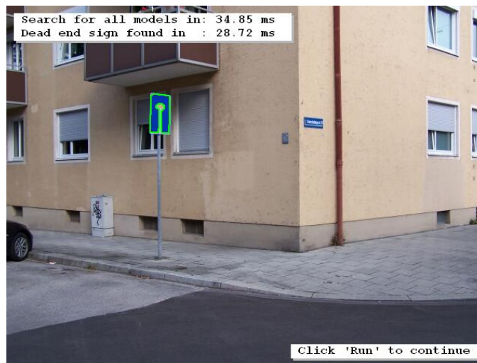
Figure 10.8: A dead end road sign is located via uncalibrated perspective deformable matching.
