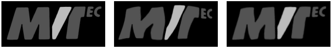
Figure 10.7: From left to right: template image, corresponding part of the search image, rectified image.
