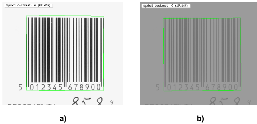
Figure 16.8: a) The bar code with a high contrast gets the grade 4 and a raw value of 82.45%. b) The defective bar code with a very low contrast gets the grade 0 and a raw value of 15.84%.
