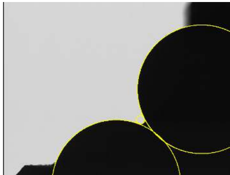
Figure 3.4: Fitting circles to the contours of the tool.
