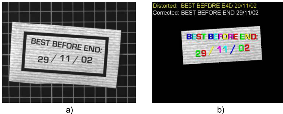
Figure 18.12: (a) Original image; (b) text is corrected using syntactic and lexicon-based auto-correction.
