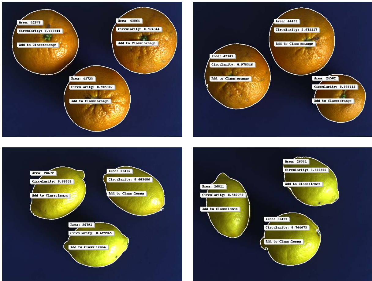
Figure 3.1: Region features of oranges and lemons are extracted and can be added as samples to the classifier.
