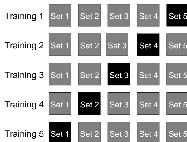
Figure 8.1: Cross validation: The training data is divided into 5 sub sets. Each set is used once as test data (black) that is classified by a classifier trained by the training data of the other 4 sub sets (gray).
