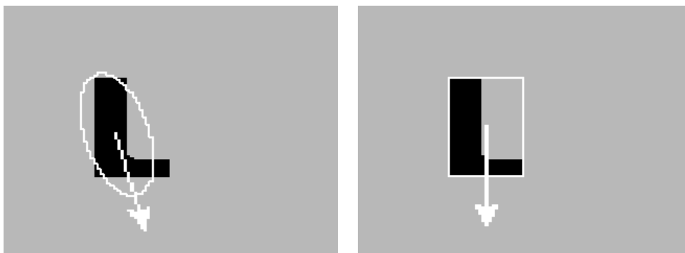
Figure 3.2: Orientation of (left) the equivalent ellipse or (right) the smallest enclosing rectangle.
