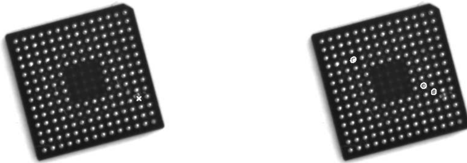
Figure 4.24: Irregularities of a BGA: (left) missing ball marked by a cross, (right) balls with center positions that deviate from the reference positions marked by ellipses.
