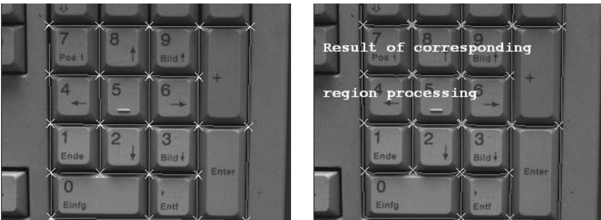
Figure 4.14: Get junction points: (left) lines fitted into linear contours and the junction points of the grid separating the keys, (right), skeleton and irregular junction points obtained by region processing.
