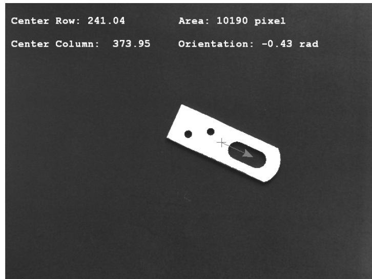
Figure 1.1: Region obtained by a threshold and display of extracted features.
